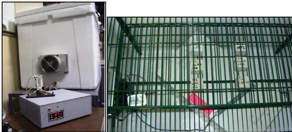
Figure 12. a) Carbonation chamber with attached heat exchanger; in the foreground is the gas control valve and temperature control module. b) A view inside the chamber; with the dehumidifier at the bottom, and the relative humidity logger on the left.
