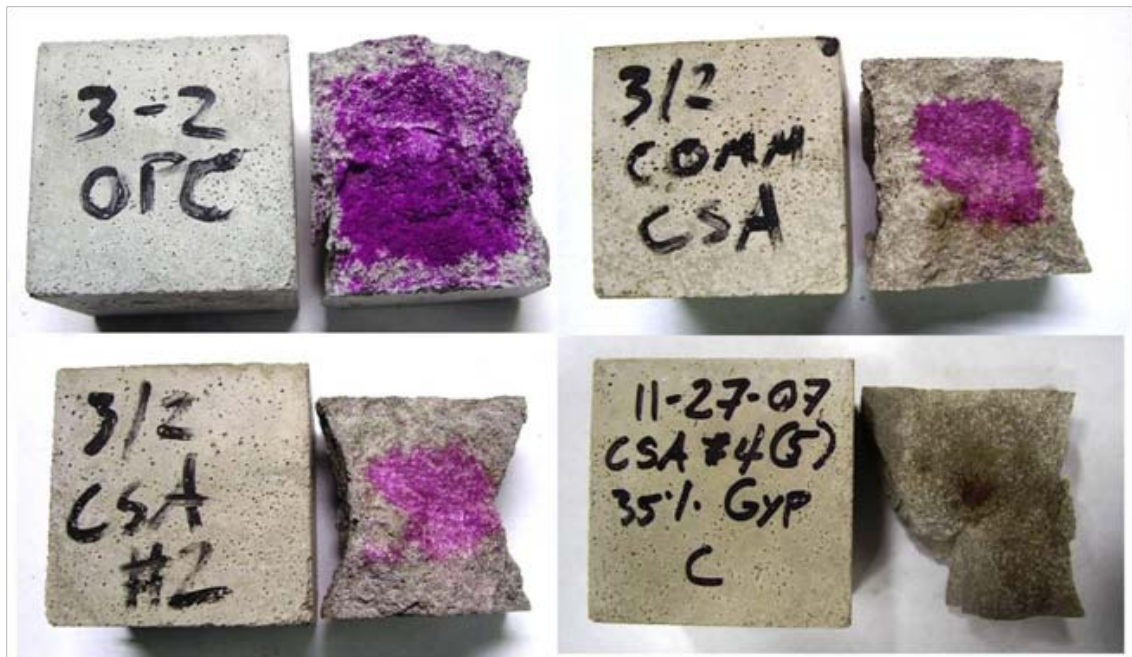
Figure 13. Mortar cubes that have been tested for compressive strength then sprayed with phenolphthalein. The rim around the pink area is the carbonation layer. These cubes have been cured for 112 days.
