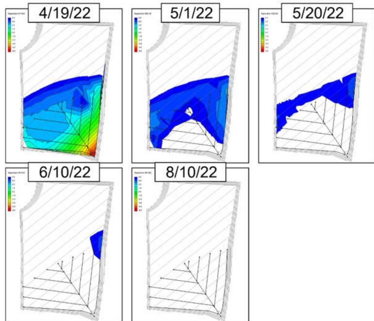
Figure 13. Groundwater separation below proposed landfill with the initial underdrain design (Linear underdrain segments shown as black lines, no color represents separation is achieved)
