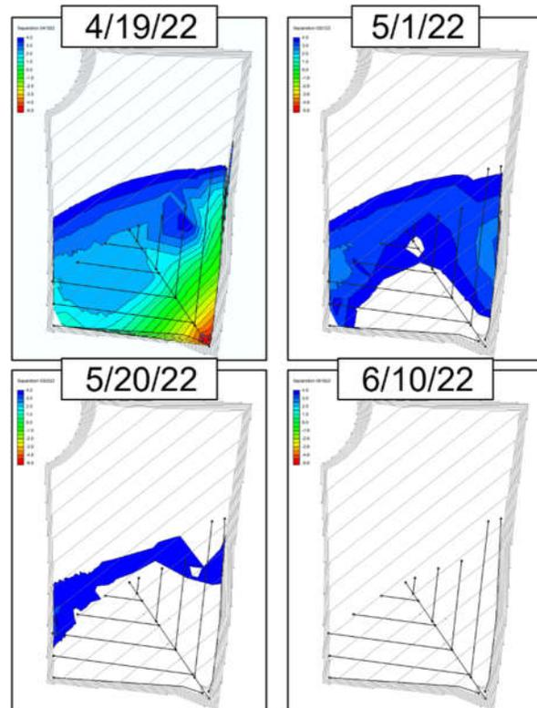
Figure 14. Groundwater separation below proposed landfill with the final underdrain design (Linear underdrain segments shown as black lines, no color represents separation is achieved)
