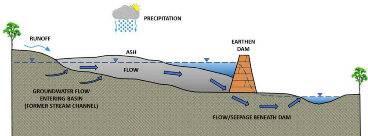
Figure 6. Revised conceptual model of the perennial stream valley CCR unit flow system
