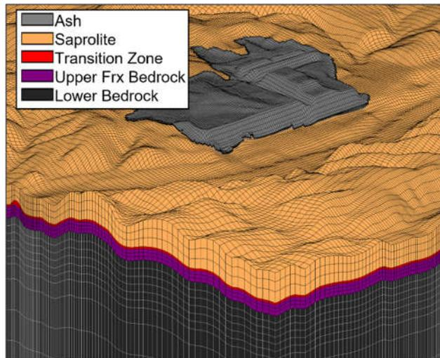
Figure 1. Flow and transport model grid
