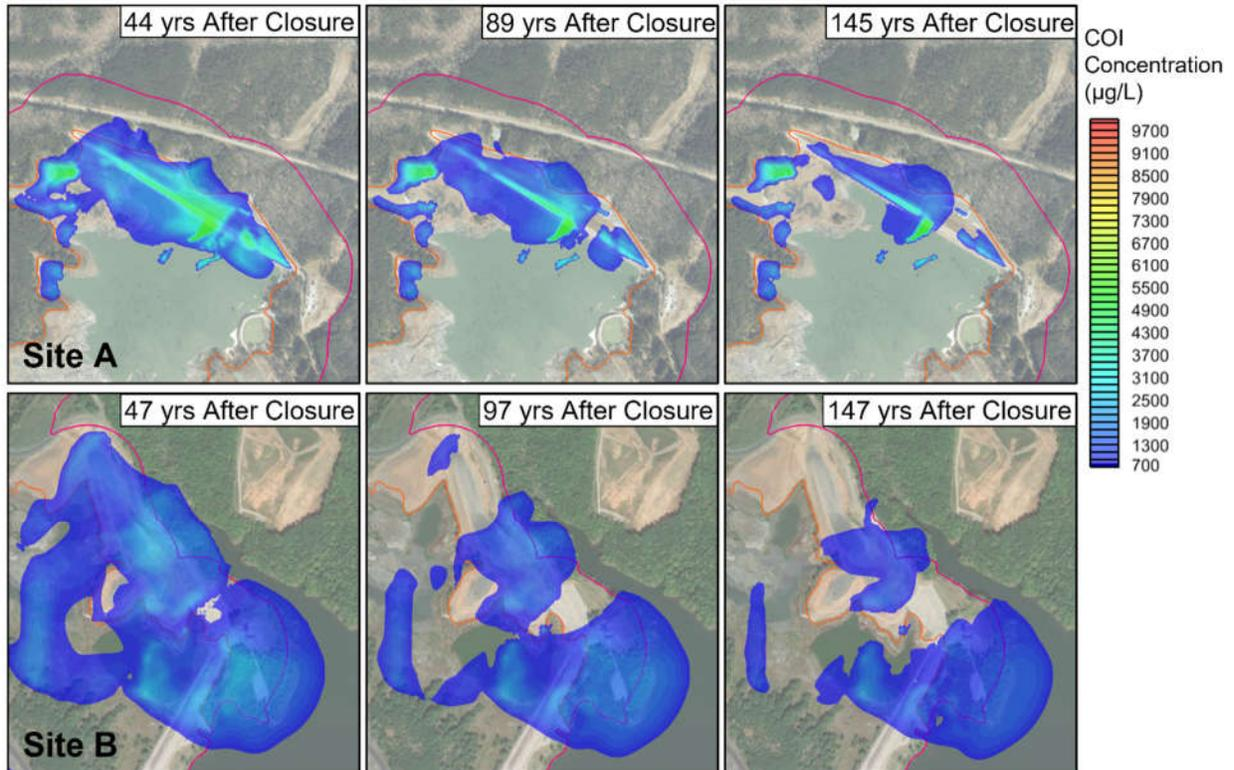
Figure 7. Comparison of predicted future boron plumes at Site A and Site B (boundary for compliance shown in pink)
