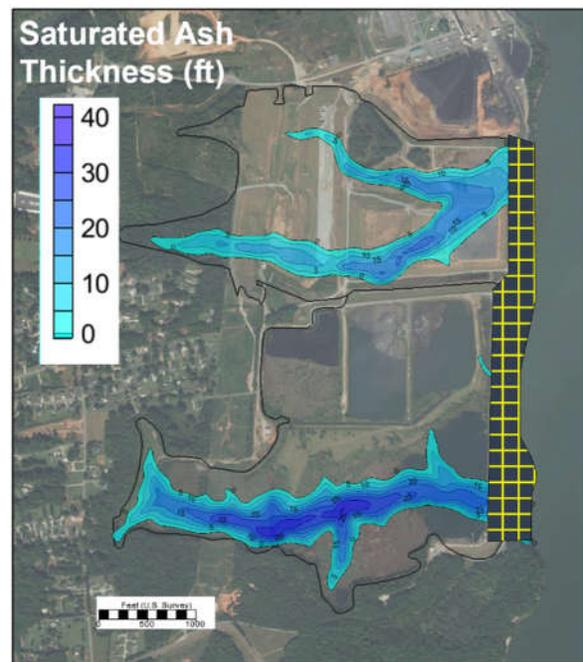
Figure 8. Estimated saturated CCR material within the CCR units under cap-in-place conditions
