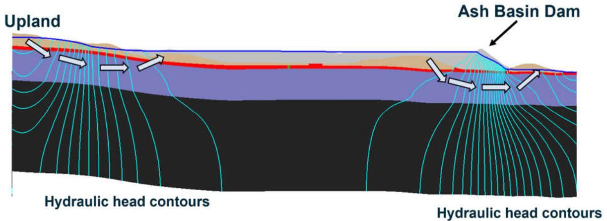
Figure 5. Modeled flow system within and below the CCR unit
