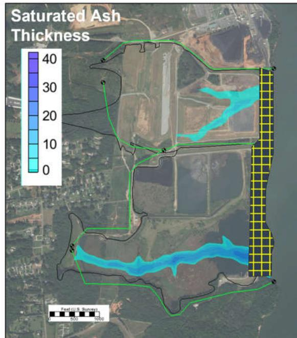
Figure 11. Estimated saturated CCR material with French drains around the periphery of CCR units under cap-in-place conditions
