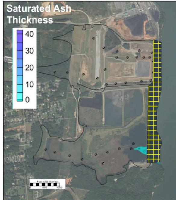
Figure 9. Estimated saturated CCR material with extraction wells below CCR material under cap-in-place conditions
