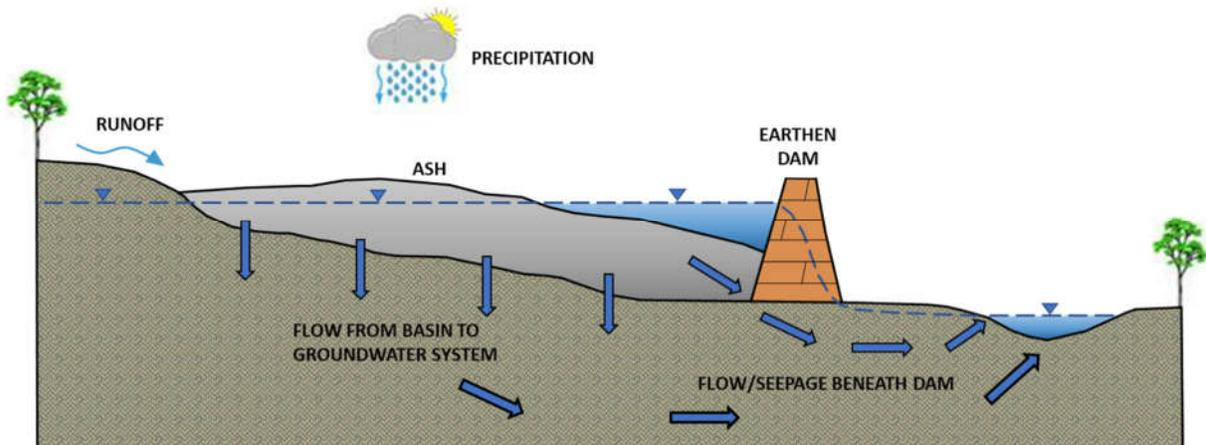
Figure 4. Initial conceptual model of the perennial stream valley CCR unit flow system
