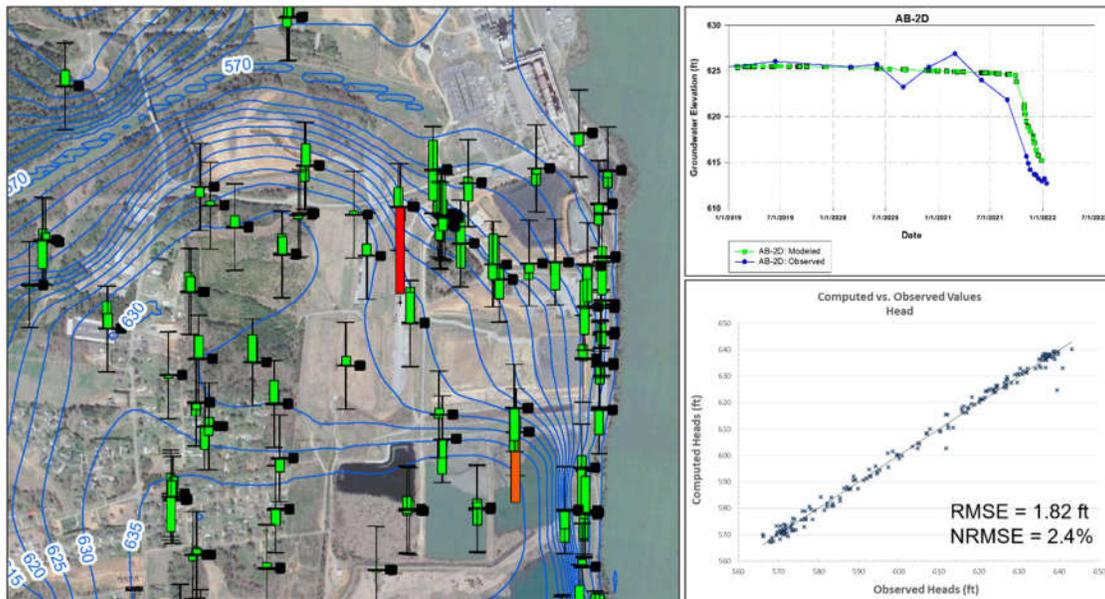
Figure 3. Flow model calibration results (error bars on plan view map show residuals between measured and predicted water levels; green: residual < 4ft, orange: 4ft < residual < 8ft, red: residual > 8ft)
