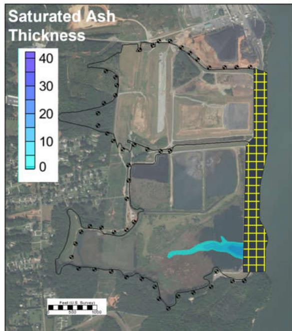
Figure 10. Estimated saturated CCR material with extraction wells around the periphery of CCR units under cap-in-place conditions
