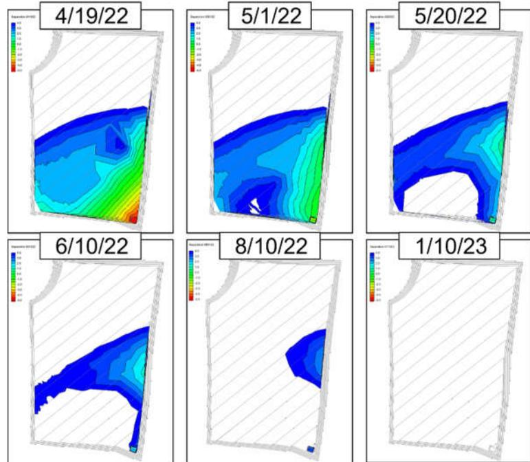
Figure 12. Groundwater separation below proposed landfill without an underdrain (No color represents separation is achieved)
