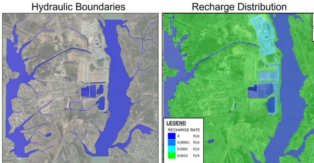
Figure 2. Hydraulic boundaries and recharge distribution model inputs
