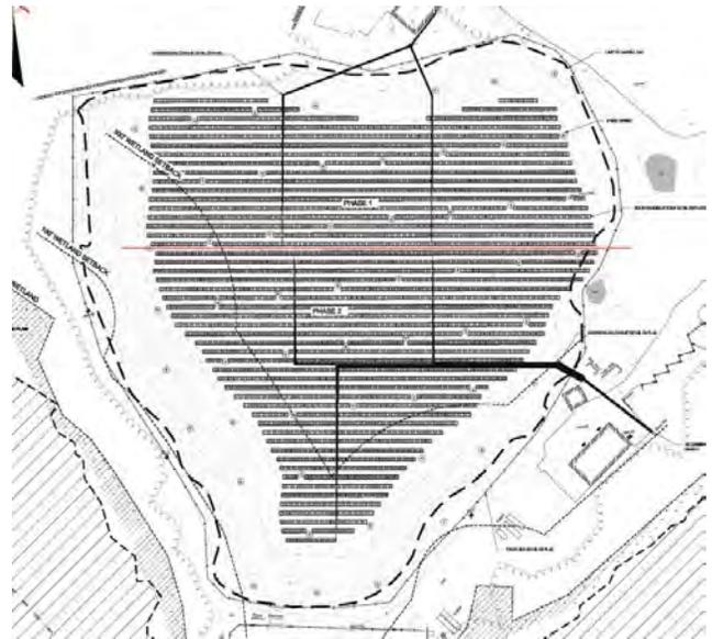
TRC additionally recommended the installation of settlement plates in the newly constructed cover system to monitor settlement. We also recommended the use of cable trays for the array wiring and modification of the stormwater conveyances to manage surface flow during peak precipitation events with the solar array in place.
