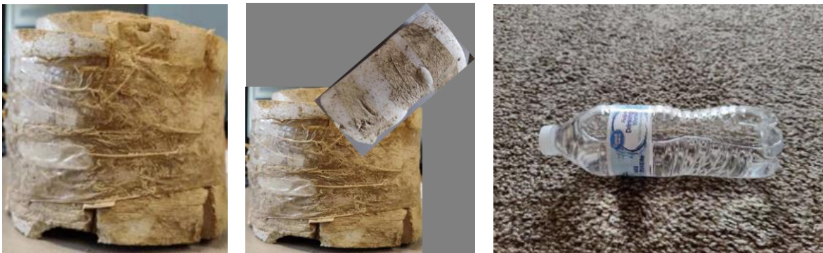
Figure 2 (Left). Styrofoam used to model a cylindrical void
