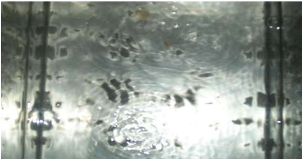
Figure 6: Appearance of the water surface in the 25 kHz ultrasonic tank; 500W (Ambedkar, 2011)
