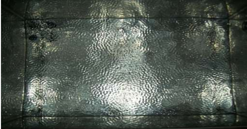
Figure 7: Appearance of the water surface in the (58/192 kHz) ultrasonic tank; 500W (Ambedkar, 2011)
