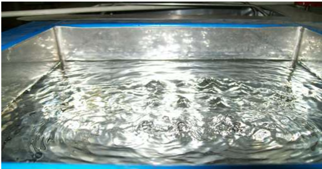
Figure 8: Appearance of the water surface in the 430 kHz ultrasonic tank; 500W (Ambedkar, 2011)
