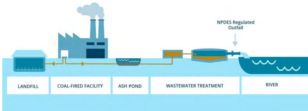
Figure 1. A coal-fired power plant facility generating CCR. CCR is disposed of in a landfill and/or surface impoundment (ash pond). Potential landfill leachate is regulated through groundwater monitoring. Ash pond wastewater is treated and discharged from a NPDES regulated outfall.
