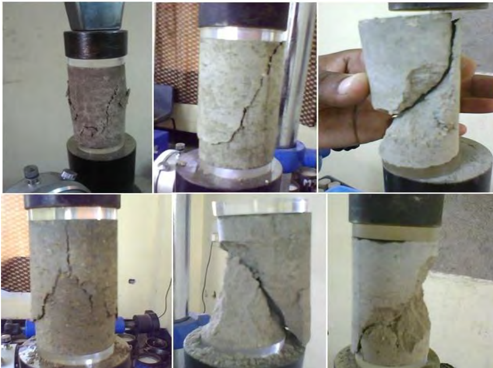
Figure 3: Post failure profiles of UCS samples
