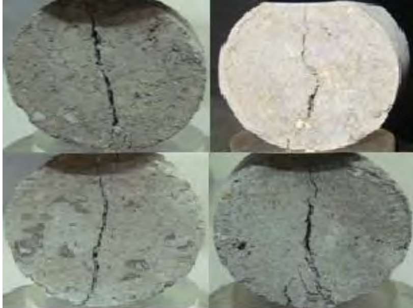
Figure 4. Post failure profiles of Brazilian tensile test samples
