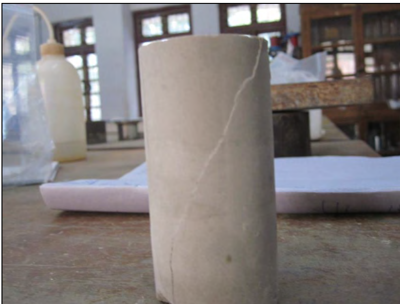
Figure 6: Post failure profile of a triaxial test specimen
