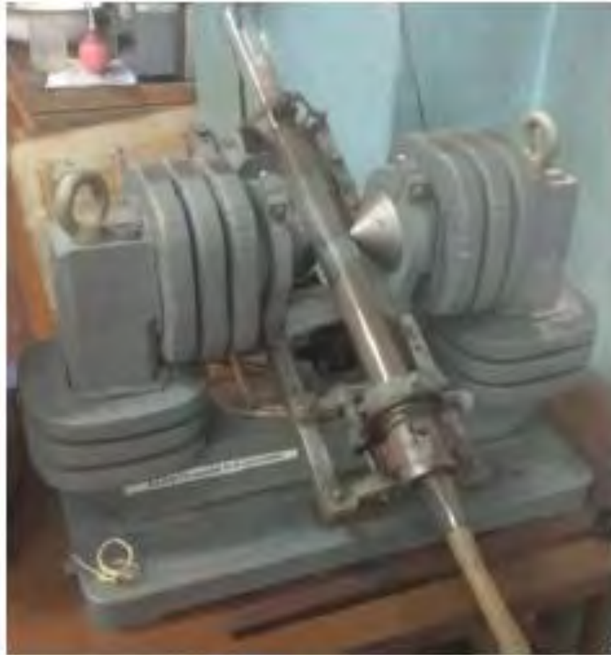
Fig. 1. Tubular magnetic analyzer 25T-SE
